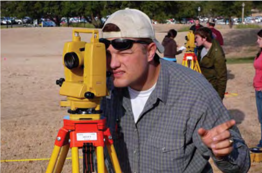
In a “mini-mester” course patterned after Auburn University’s highly successful surveying camp, Texas A&M construction science students learn construction surveying techniques using tripods, grade rods, transits and total stations.
