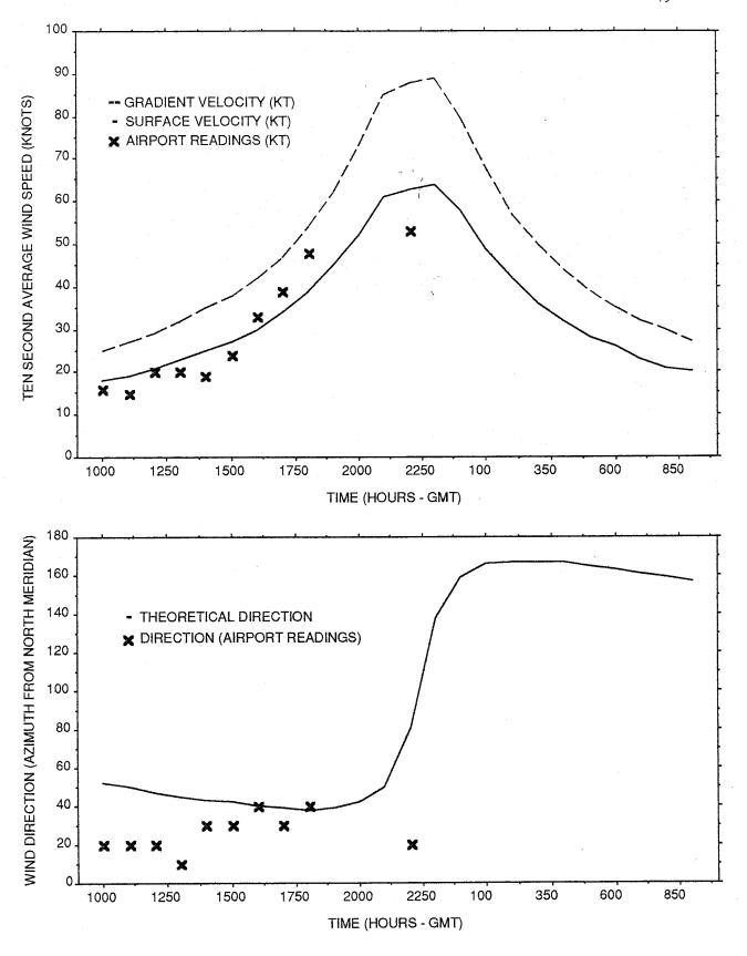
Figure 4. Comparison Between Predicted Wind Velocity Measured Wind Velocity at Montago Bay Airport
