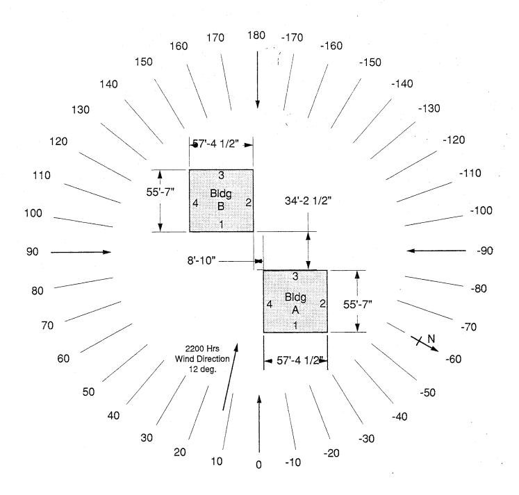
Figure 9. Layout of Wind Tunnel Test
