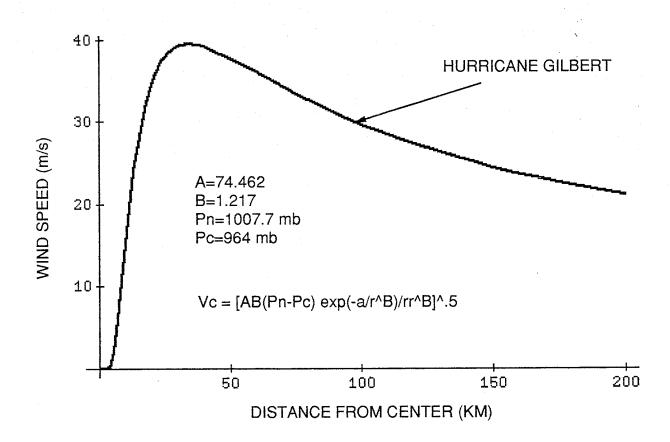
Figure 3. Windspeed Profile of the Calibrated Hurricane Model
